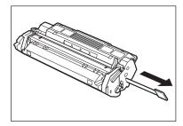
**7** Hold the cartridge and position the arrow mark on the cartridge towards the inside of the machine shown below.
