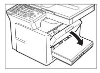
**2** Remove the cartridge from the machine.
