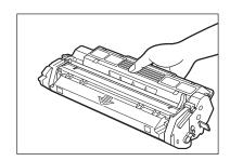
**8** Align the projections (a) on both sides of the cartridge to the guides (b) in the machine (location (1)) and gently slide the cartridge into the machine until the right cover slightly rises up (location (2)).
