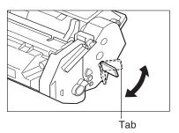
**6** While grasping the cartridge with one hand, firmly and slowly pull the sealing tape tab with the other hand to remove the sealing tape completely. Throw the tape away.
