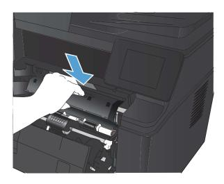
Installation is complete. Place the used toner cartridge in the box in which the new cartridge arrived. See the enclosed recycling guide for recycling instructions.
