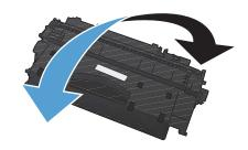
Bend the tab on the left side of the cartridge until the tab breaks loose. Pull the tab until all the tape is removed from the cartridge. Place the tab and tape in the toner cartridge box to return for recycling.
