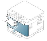
3. Grasp the handles on the toner cartridge and pull to remove the cartridge from the machine.
