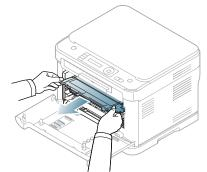
4. Pull the waste toner container out of the machine using its handle.
