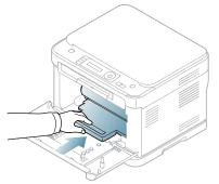
8. Insert the waste toner container into position and then push it to make sure that it is firmly seated in place.
