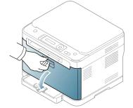
**3.** Grasp the handles on the front cartridge and pull to remove four cartridges from the machine.
