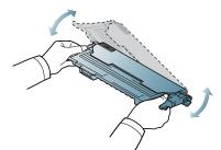
7. Place the toner cartridge on a flat surface as shown below and remove the protecting cap.
