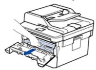
4. Push down the green lock lever and take the toner cartridge out of the drum unit.
