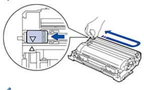
Be sure to return the tab to the Home position (**\( \Lambda \)**). The arrow on the tab must be aligned with the arrow on the drum unit. If it is not, printed pages may have a vertical stripe.
