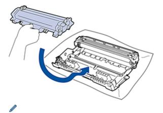
Make sure you put the toner cartridge in correctly or it may separate from the drum unit.
