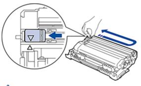
Be sure to return the tab to the Home position ( $\blacktriangle$ ). The arrow on the tab must be aligned with the arrow on the drum unit. If it is not, printed pages may have a vertical stripe.
