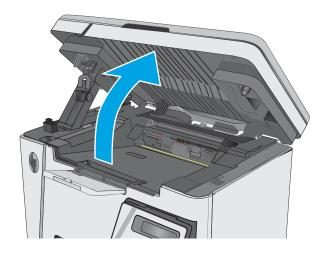
2. Remove the used toner cartridge from the printer.
