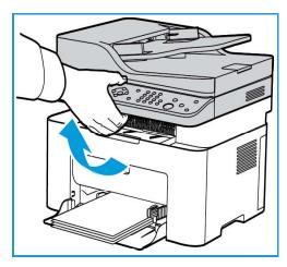
2. Reach in where the arrow indicates 'open' on the right and pull up to release the inside cover. Then lift the panel in the center of the machine to reveal the print cartridge.
