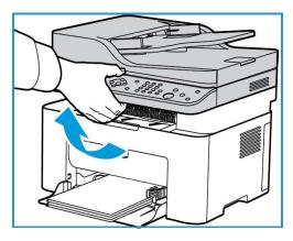
2. Reach in where the arrow indicates 'open' on the right and pull up to release the inside cover. Then lift the panel in the center of the machine to reveal the print cartridge.
