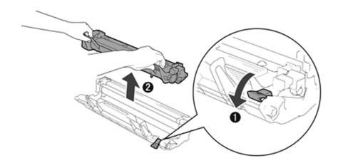
5. Unpack the new drum unit and put the toner cartridge firmly into the new drum unit until you hear it lock into place. If you put the cartridge in correctly, the lock lever on the drum unit will lift automatically.
