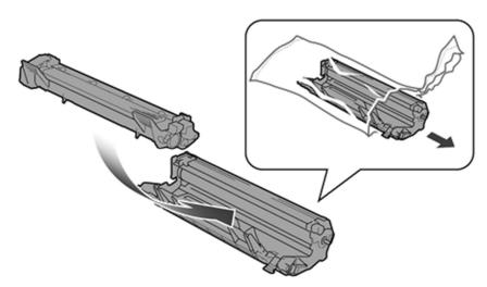
5. Put the drum unit and toner cartridge assembly back into the machine. Do not close the top cover yet.
