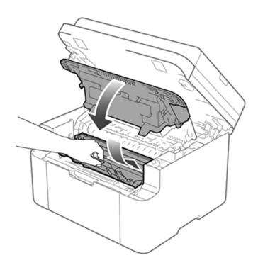
7. After pulling the pull-arm (2) on the left side of the machine down, close the scanner cover.
