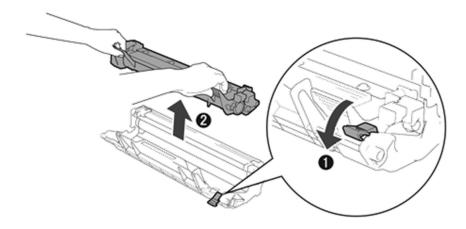
4. Unpack the new drum unit and put the toner cartridge firmly into the new drum unit until you hear it lock into place. If you put the cartridge in correctly, the lock lever on the drum unit will lift automatically.
