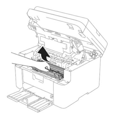
4. Push down the lock lever (1) and take the toner cartridge out of the drum unit (2).
