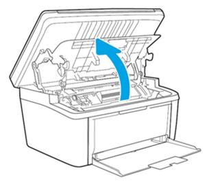
2. Grasp the handle on the toner cartridge, and then pull the toner cartridge out to remove it.
