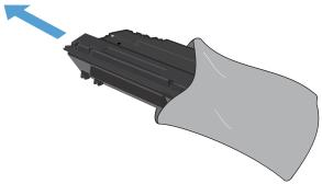
Grasp the front and back of the toner cartridge, and distribute the toner by gently rocking the toner cartridge five or six times.
