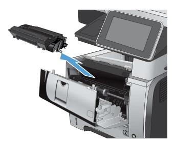
4. Remove the new toner cartridge from the bag. Place the used toner cartridge in the bag for recycling.
