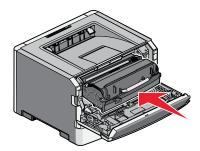
8 After you replace the photoconductor kit, reset the photoconductor counter.
