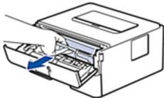
4. Push down the green lock lever, and then take the toner cartridge out of the drum unit as shown in the illustration.
