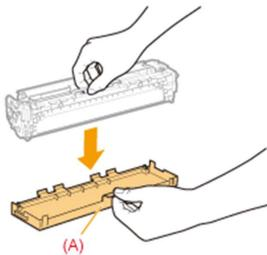
9. Install the toner cartridge. Be careful not to let the drum impact the frame of the toner cartridge tray.
