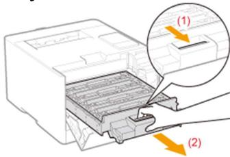
3. Hold the toner cartridge to be replaced by its handle and pull it straight up and out of the printer.
