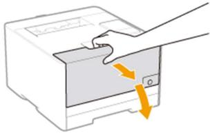
2. Press the lever and pull out the toner cartridge tray.
