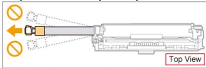
If the sealing tape stops at midpoint, pull it out of the toner cartridge completely.
