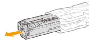
5. Shake the toner cartridge five or six times as shown in the figure to evenly distribute the toner inside the cartridge. Do not remove the drum protective cover (A).
