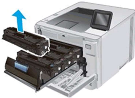
Figure : Removing the toner cartridge
