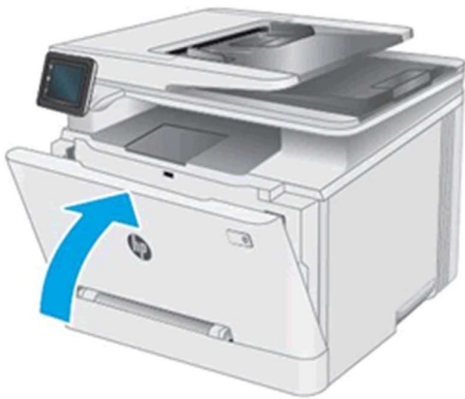
Figure : Closing the toner cartridge drawer
