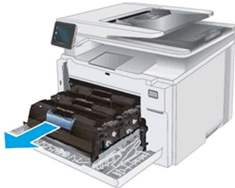
Figure : Pulling out the toner cartridge drawer
