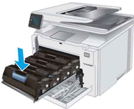
Figure : Inserting the toner cartridge into the printer
