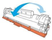
5. Bend the tab on the toner cartridge, and then pull the tab until all the sealing tape is removed from the toner cartridge.
