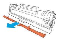
7. Align the new toner cartridge with the tracks inside the printer, and then push the toner cartridge until it is firmly seated.
