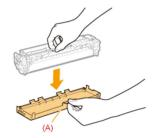
9. Install the toner cartridge. Be careful not to let the drum impact the frame of the toner cartridge tray.
