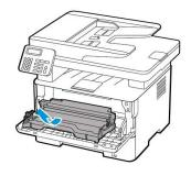
3. Remove the used toner cartridge from the imaging unit.
