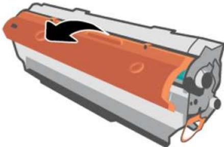
4. Grasp the cartridge by its sides, and then rock the cartridge side to side five or six times to evenly distribute the toner.
