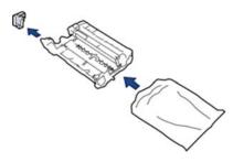
7. Push the toner cartridge firmly into the new drum unit until it locks into place.
