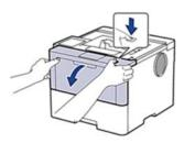
3. Remove the toner cartridge and drum unit assembly from the machine.
