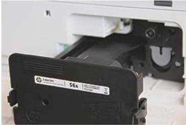
2. Remove the replacement toner cartridge from its packaging. Save all packaging for recycling the used toner cartridge.
